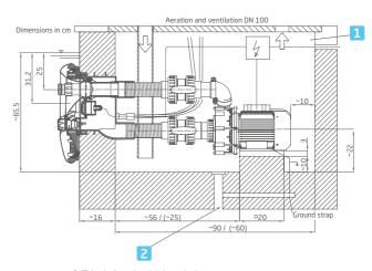
Sufficiently dimensioned drain required
